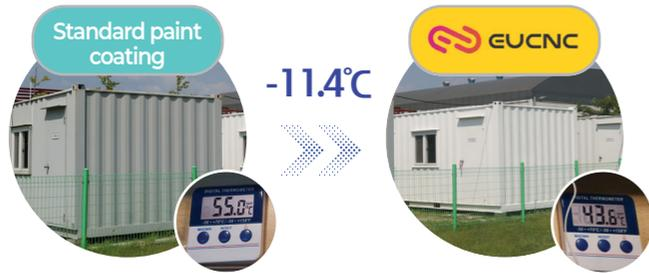
In a pilot test conducted at our Incheon headquarters, the general paint reached 55°C, while EUCNC paint maintained a lower temperature of 43.6°C, demonstrating a difference of 11.4°C.
